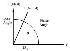
In practice the current leads the voltage by some other phase angle due to the series resistance R<sub>s</sub>. The complement of this angle is called the loss angle and:
