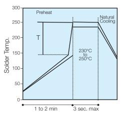
(Preheat chips before soldering) T/maximum 150°C
