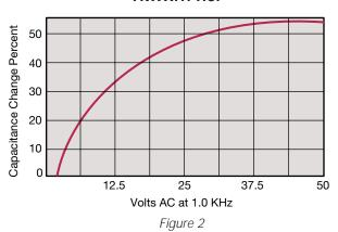
Capacitor specifications specify the AC voltage at which to measure (normally 0.5 or 1 VAC) and application of the wrong voltage can cause spurious readings. Figure 3 gives the voltage coefficient of dissipation factor for various AC voltages at 1 kilohertz. Applications of different frequencies will affect the percentage changes versus voltages.
