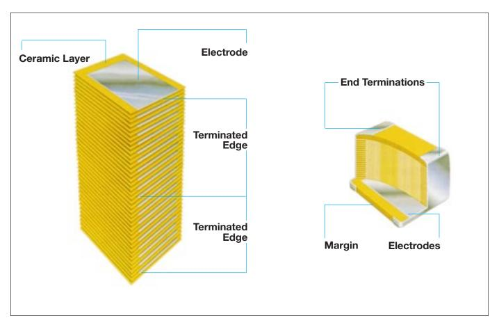
**Formulations -** Multilayer ceramic capacitors are available in both Class 1 and Class 2 formulations. Temperature compensating formulation are Class 1 and temperature stable and general application formulations are classified as Class 2.
