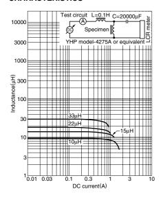
Test equipment L: 4194A IMPEDANCE/GAIN-PHASE ANALYZER HP, or equivalent (Test frequency: 100kHz/0.5V)
